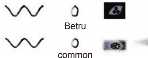
Pre-deformation steel cords used to improve tyre strength and durability
